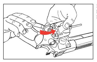
FIGURE 3 LOADING THE REVOLVER.
