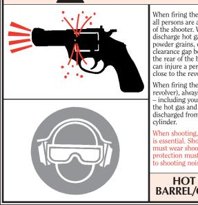
When firing the GP100 revolver, be sure all persons are a safe distance to the rear of the shooter. When fired, all revolvers discharge hot gas and particles of lead, powder grains, or lubricant through the clearance gap between the cylinder and the rear of the barrel at high speed. This can injure a person who is standing too close to the revolver.
