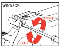
To move the point of impact to the <u>right</u>: turn screw <u>counterclockwise</u>.
