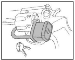
Correct Installation of Lock For Ruger GP100<sup>®</sup> Revolvers <u>Only</u>
